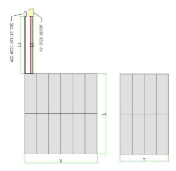
T: 87mm W: 131mm L: 150mm L1: 100mm L2: 100mm
