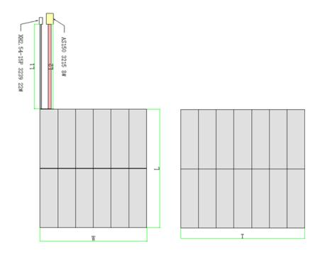
T: 152mm W: 129mm L: 150mm L1: 100mm L2: 100mm
