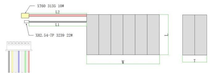
T: 45mm W: 131mm L: 80mm L1: 100mm L2: 100mm
