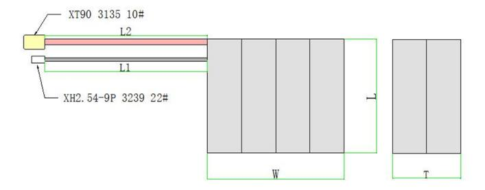
T: 45mm W: 89mm L: 80mm L1: 100mm L2: 100mm
