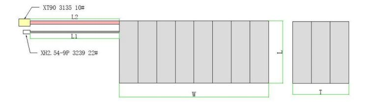
T: 66mm W: 173mm L: 80mm L1: 100mm L2: 100mm
