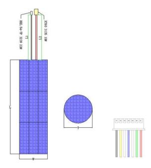
T: 73mm W: 73mm L: 230mm L1: 100mm L2: 100mm
