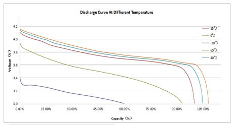
Charge CC ,CV:0.5C,4.2V;0.02C cut off @25°C Discharge CC:0.5C ;3.0V cut off @25°C
